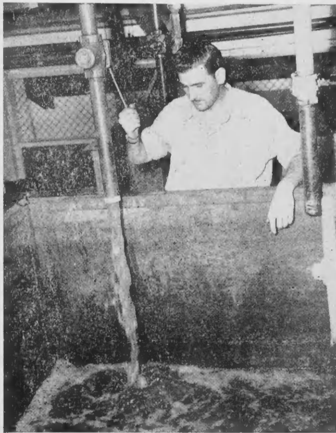
Aloe juice is charged into one of the tanks which separate out the plant resins and other impurities. After further chemical processing, the pure aloin is derived and dried in a large oven.
